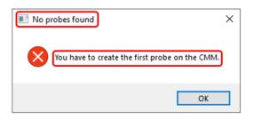
After confirming this message with OK, the software is closed and a probe must be created in PC-DMIS.
