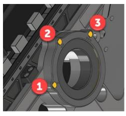
The sequence of the countersinks is visualized in PC-DMIS.
